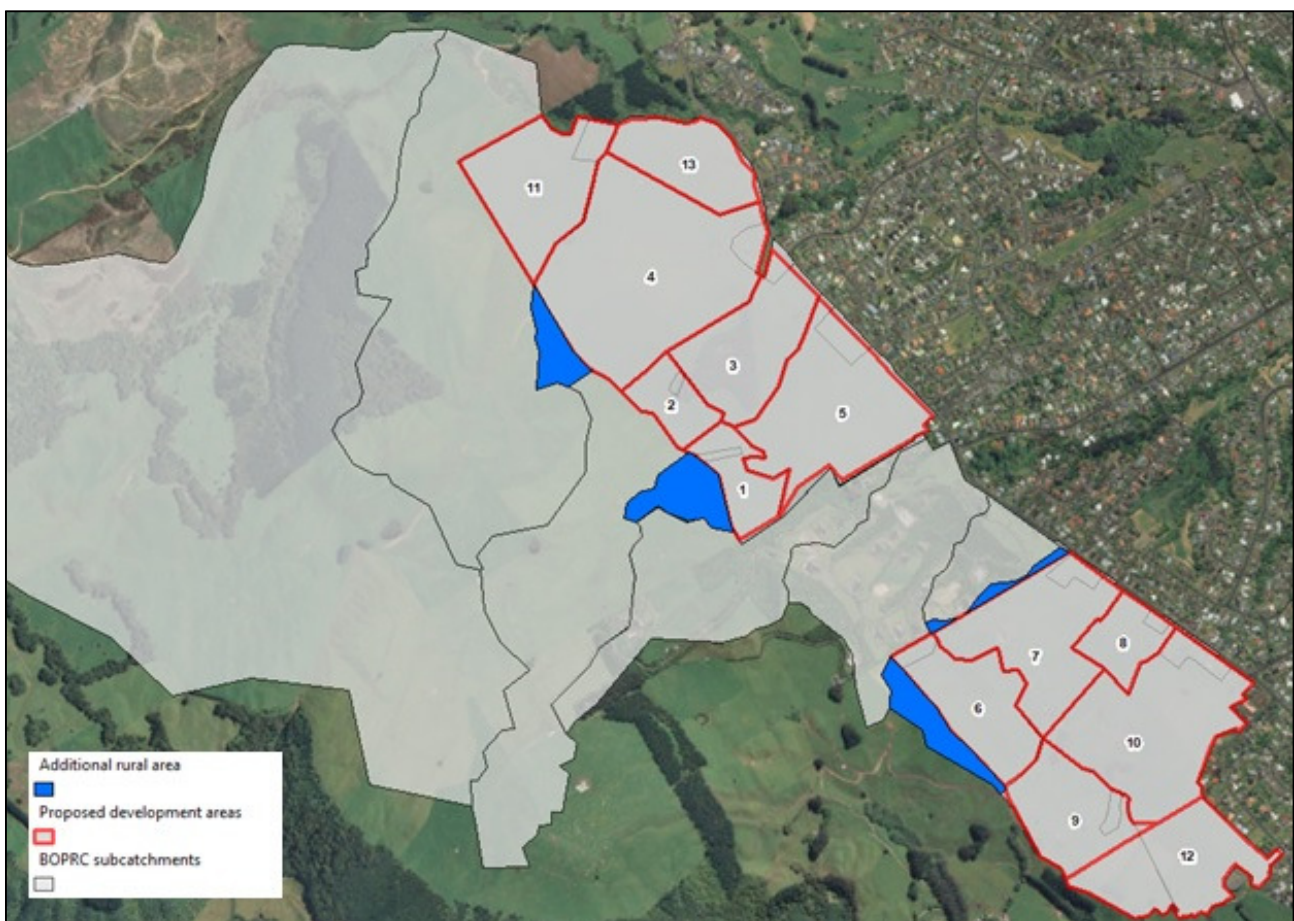
Figure 2-5: Subcatchment amended to represent the Proposed development (blue areas identify areas outside the proposed development that are currently incorporated into the stormwater management approach).
